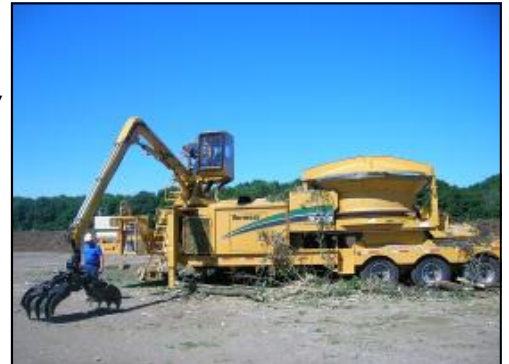
A tub grinder from Northeast Indiana Solid Waste District that would be used for grinding debris during a natural disaster.
